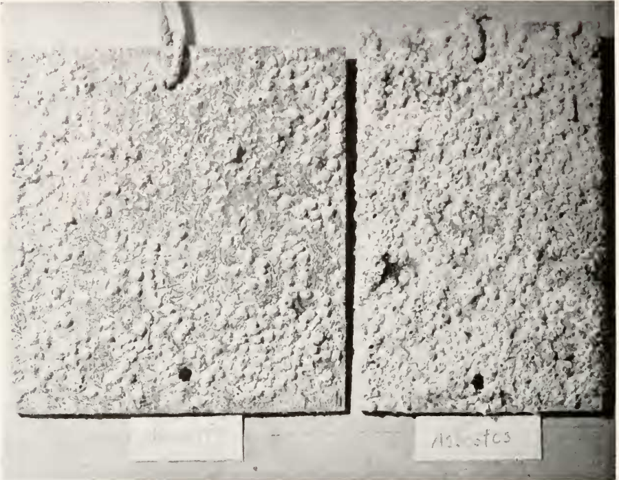
FIGURE 2. Accumulation of fouling organisms on masonite and asbestos after 90 days' exposure at Belle Isle, Miami Beach, Florida.
